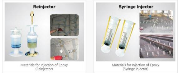
(1) Reinjector is a mid-low pressure injecting device, upgraded to improve the effectiveness of grouting for crack repairing by incorporating the merits of the high pressure grouting of packer and the merits of syringe injector.
